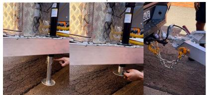
• Attach safety chains to vehicle ensuring they cross over each other. Attach light cable and release the hand brake. Check all lights on the trailer are working.
