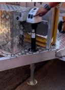
• Continue to retract the stabiliser leg all the way to the top. Once it cannot travel any further, remove the pin from the leg itself and push it up. Put the pin back into the bottom holes and secure the pin latch.
