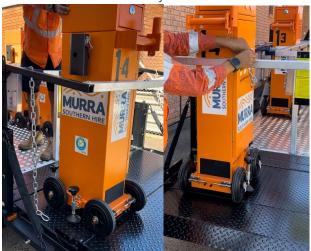
• Locate rear control panel. Press circular power button once. After 5 seconds press the white logo twice to activate. Both lights should turn on
